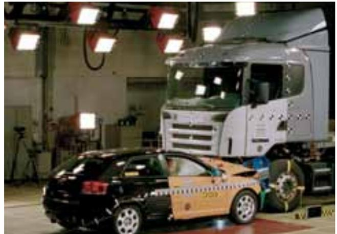
Front underrun protective devices assist in activating safety features in cars
