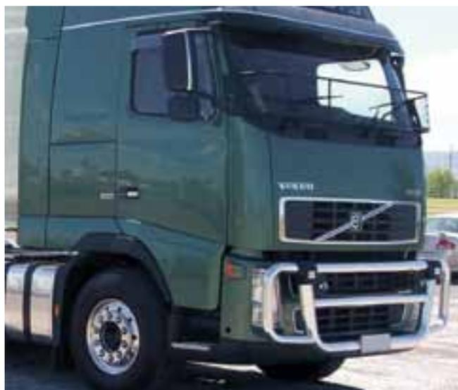
A current example of a bullbar that does not interfere with the integrated energy absorbing FUPD
