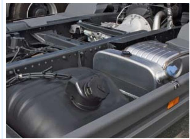
Vehicles fitted with Selective Catalytic Reduction emission technology may require an Adblue™ tank or tank for urea
