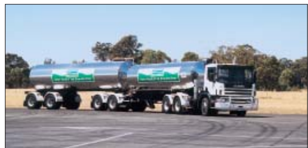
Mini B-doubles are more manoeuvrable than conventional semi-trailers
